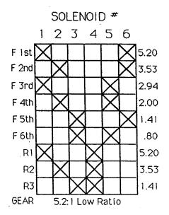
To troubleshoot the electric circuit of the valve, the above charts show what solenoids are charged when that gear is selected. The transmission ratio must be known.
