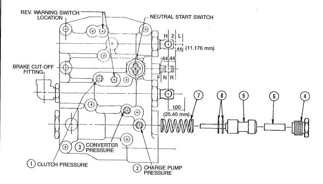
The pressure checks are to be made with the transmission oil temperature at 170° or (76.7°C) to 185°F. (85°C)
