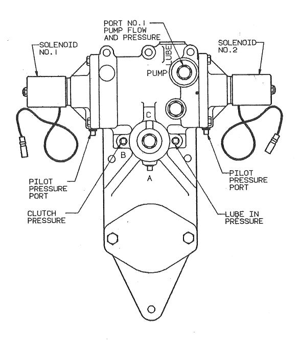
FOR SINGLE PRESSURE APPLIED CLUTCH
